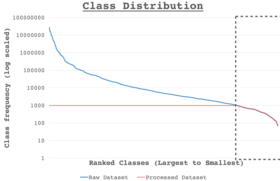
Figure 4.4: Distribution of classes. (Blue) shows the distribution of our dataset before K -means clustering was used; (Red) shows the distribution after running K -means clustering on classes with more than 1,000 datapoints.
