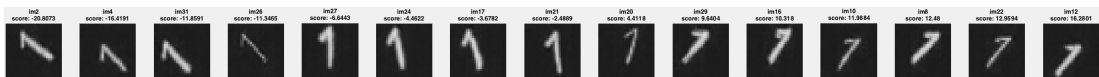
Figure 4.5: Using 1000 latent variables sampled from the normal distribution, we generate 1000 new images with the Digits GAN. 1000 scores can therefore be computed. From the sorted scores, we pick 15 samples and display their corresponding image.
